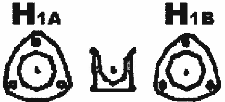
FIGURE 2. 13,800GRD Y/7970 V Loop Feed Bushing Configuration
